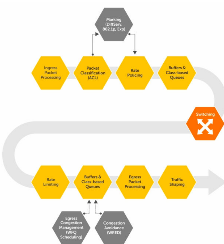
Figure 104. Dell Networking QoS Architecture
